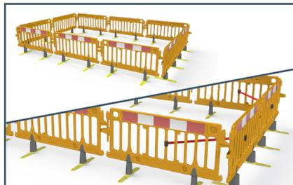
2. Place the Avalon Barrier in a box formation, connecting them with the hook and bucket system. Optional Stability Bars can be added to reduce the risk of barriers sliding & folding into each other.
